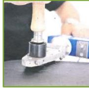
11. Screw the welding plug onto the handle of the heating element to 250°C +/- 10°C. With a light pressure both joint and welding plug are heated at the same time.
